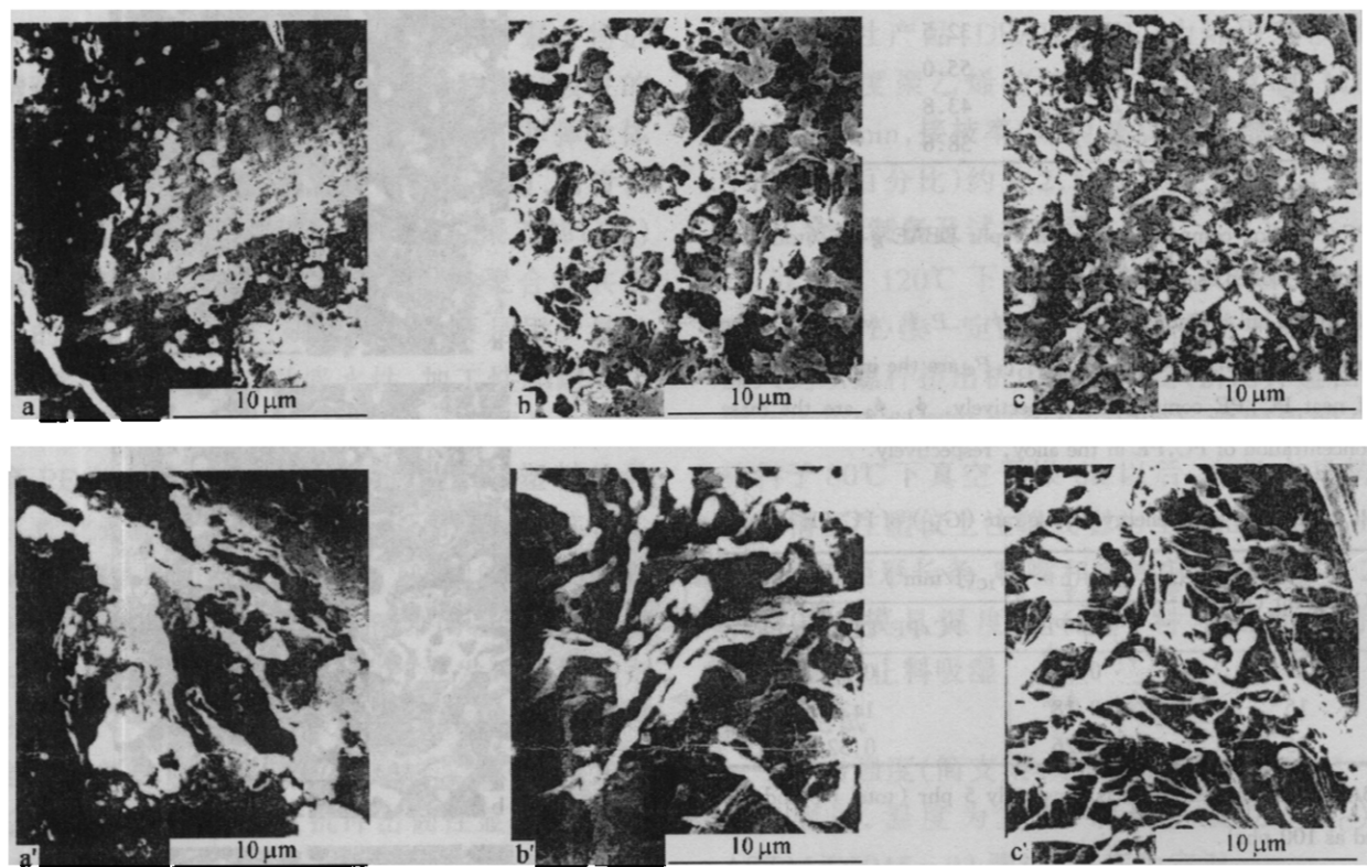
Fig. 2 Scanning electron micrograph of the fracture surface of the PC/PE alloy compatibilized with 5 phr DBAE- g -PE a, b and c: the surfaces obtained from frozen fracturing in liquid nitrogen; a', b' and c': the surfaces obtained from impact fracturing at room temperature; the PC content is 5 phr (a and a'), 15 phr (b and b'), 35 phr (c and c').
